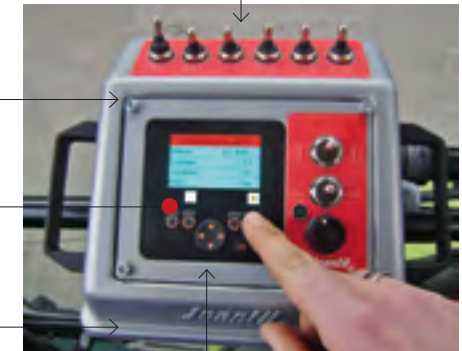
Spreading setting on SMART Control display (e.g. 10 t/ha, actual spreading width 12 m)
